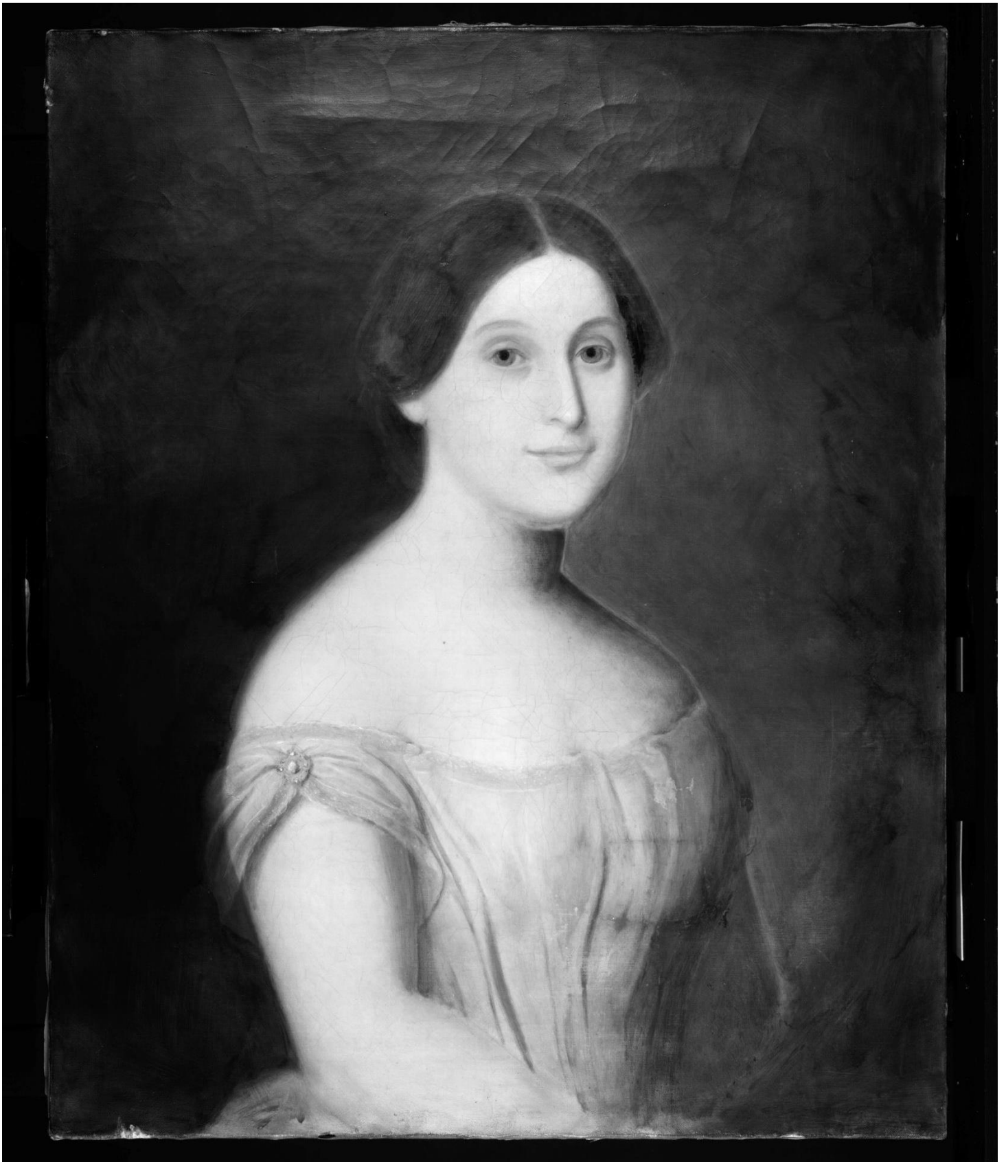
Figure 11. Infrared reflectography. Apollo Camera by Opus Instruments (900-1700 nm). Apollo 1.1.4.0 software. Two Lowel Tota-Lite Tungsten flood lights, at a 45-degree angle. 30 milliseconds integration time. No filter.
